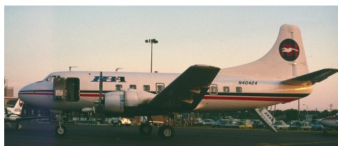
Provincetown Boston Airlines 4-0-4 displaying its characteristic tail passenger ramp
